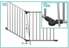
Reinstall a removable, vertical bar. Insert bar by pressing it into upper hinge cone, while sliding bar into groove of lower hinge. Spring in cone will make bar lock in place. Proceed to "Installation" steps 13 to 23.
